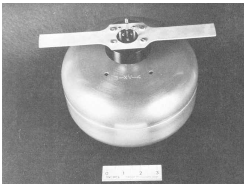
FIG. 2. Completely assembled B-XV rotor with removable upper seal in place.
